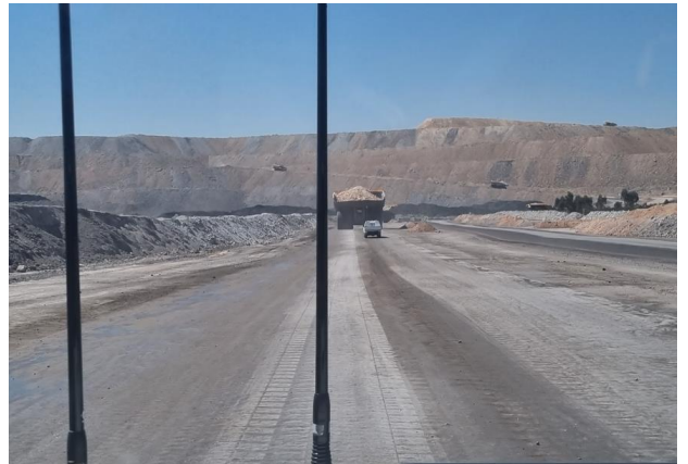
Photograph 17: Haulage road with water to reduce dust
