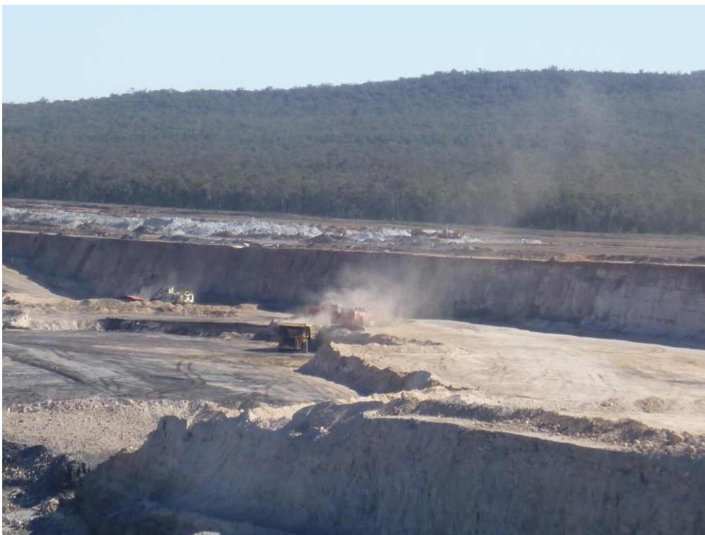
Photo 2 – Dust generation from truck and shovel
