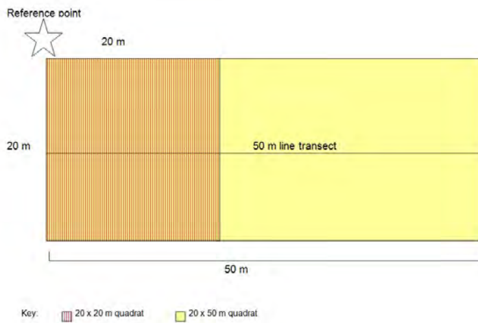
Figure 4-1 Schematic diagram illustrating the layout of the nested 20 x 50 m and 20 x 20 m quadrats used for the assessment of condition attributes at each site
