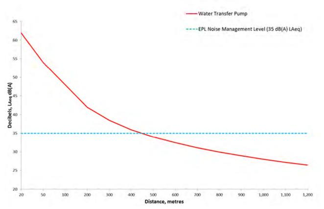
Figure 6.8 Estimated noise levels at increasing separation distance from the pump
