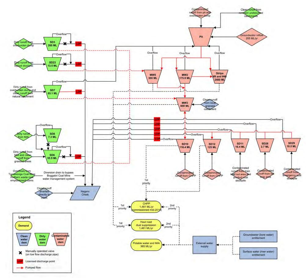
**FIGURE 2B** WATER BALANCE MODEL SCHEMATIC - YEAR 2015 (JULY TO DECEMBER 2015)
