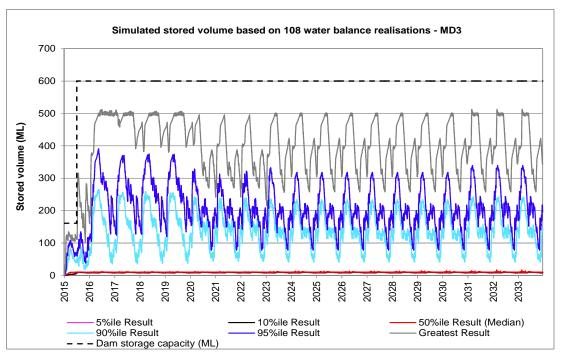
Figure 4.5 Simulated time series of water stored in MW3
