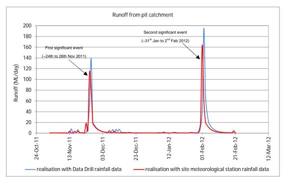
Figure 4.7 Simulated contaminated runoff generated for pit catchment from 1 November 2011 to 21 February 2012 – model verification
