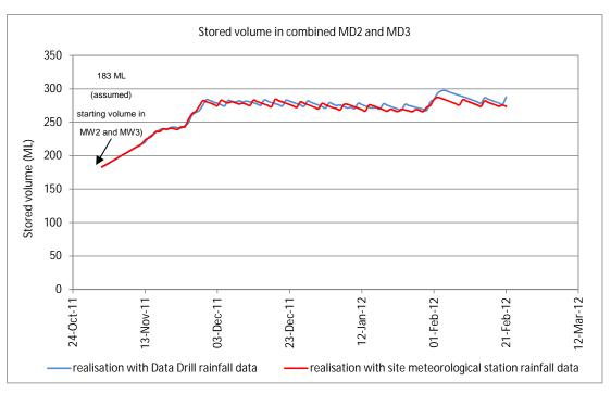
Figure 4.9 Simulated volume of total water stored in MWDs (MW2 and MW3) from 1 November 2011 to 21 February 2012 – model verification
