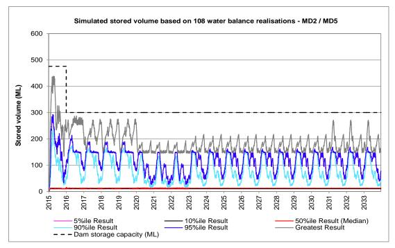
Figure 4.4 Simulated time series of water stored in combined MW2 and MW5
