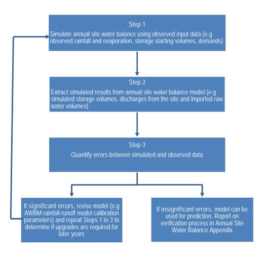
Figure 6.1 Water balance model verification process
