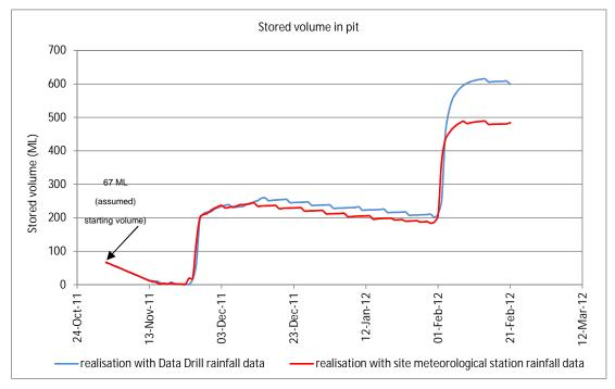
Figure 4.8 Simulated volume of water stored in-pit from 1 November 2011 to 21 February 2012 – model verification
