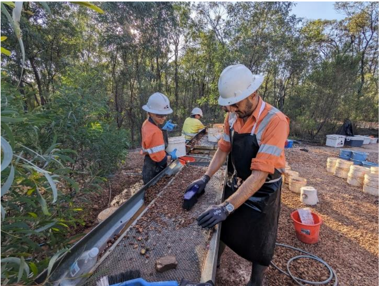
Figure 6.9: Wet Sieving being undertaken in 2023 at BC 54
