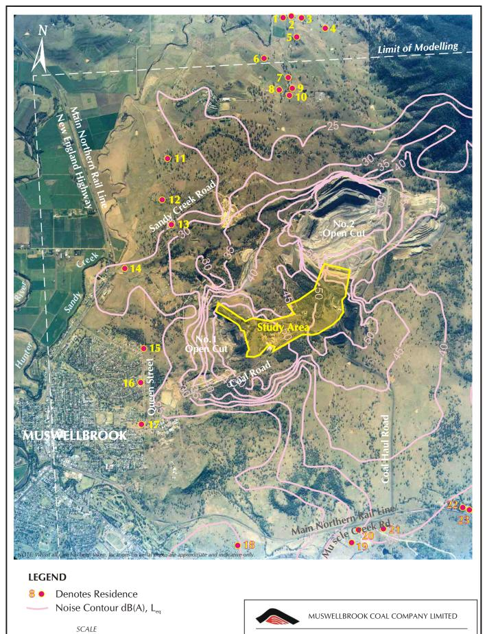
Noise Contours: Year 1 - Excavator at Ground Level Above No.1 Open Cut Highwall NW Wind FIGURE 6.5
