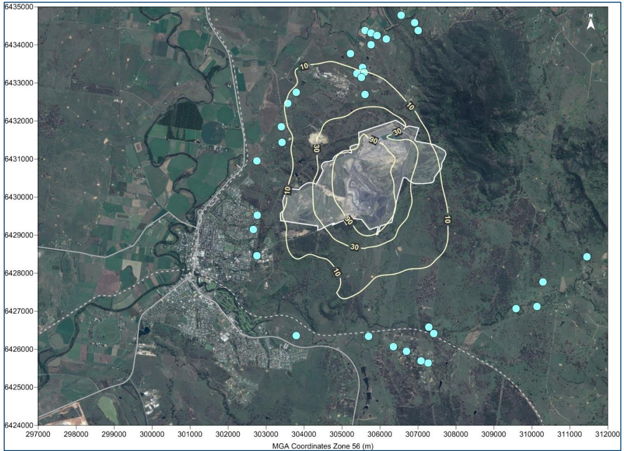
Figure E-6: Predicted annual average TSP concentrations due to emissions from the modification in 2017 ( \mu\text{g}/\text{m}^3 )
