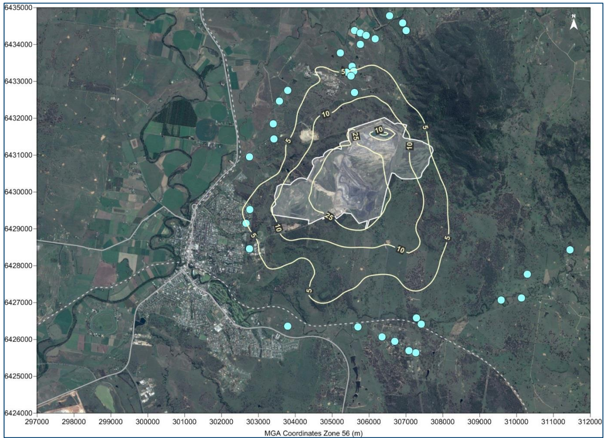
Figure E-1: Predicted maximum 24-hour average PM 2.5 concentrations due to emissions from the modification in 2017 (µg/m 3 )
