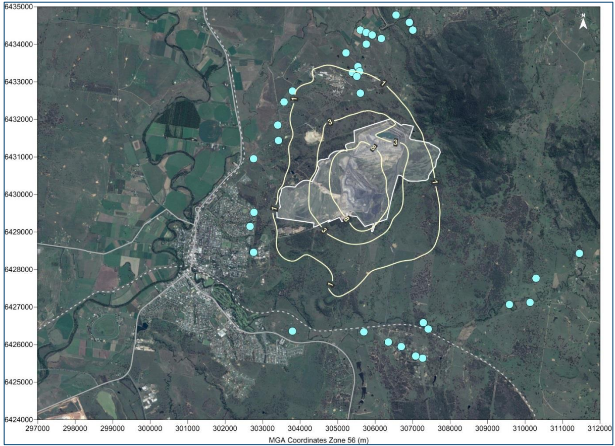
Figure E-2: Predicted annual average PM 2.5 concentrations due to emissions from the modification in 2017 ( \mu\text{g}/\text{m}^3 )
