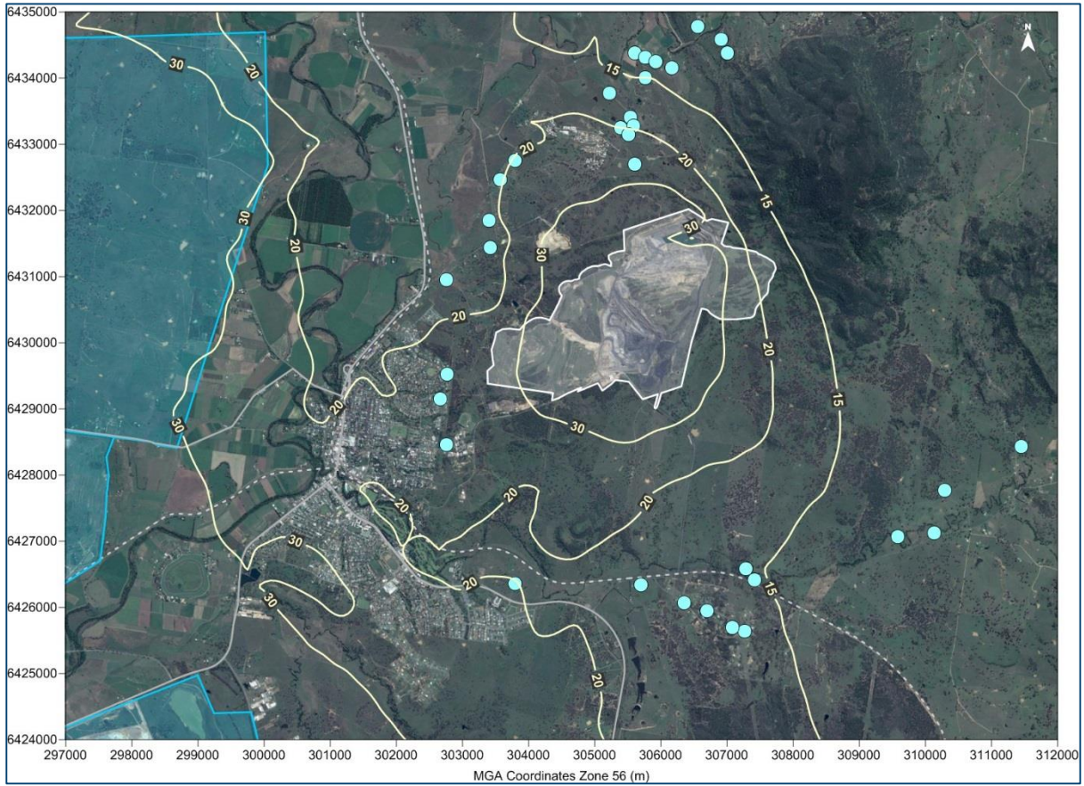
Figure E-5: Predicted annual average PM 10 concentrations due to emissions from the modification and other sources in 2017 (µg/m 3 )
