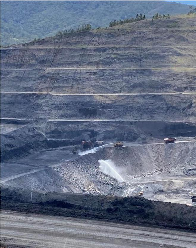
**Photo 3 – Water carts located in Open Cut Mine 1 controlling minor spontaneous combustion**
