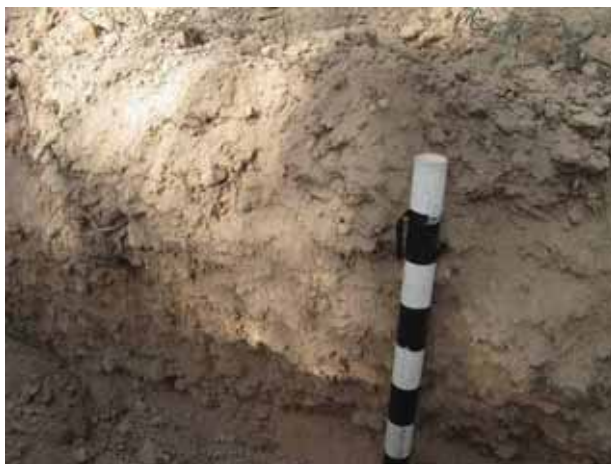
Plate 3 – Light Brown Uniform gravelly Sand Profile
