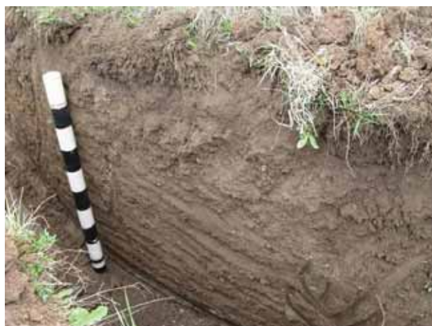
Plate 7 – Brown Gradational Clay Profile
