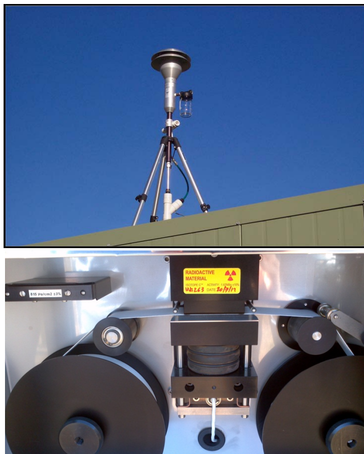
Figure 12 - TEOM PM 10 MONITOR (top) and BAM PM 10 MONITOR
