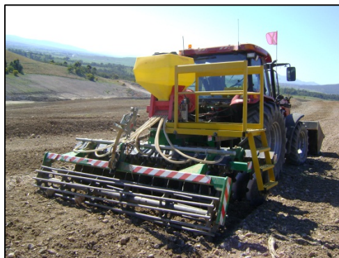
Figure 64 - Air Assisted Planter for Tree Seeding
