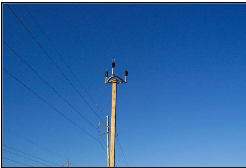
Figure 54- REAL TIME NOISE MONITORING MICROPHONE ASSEMBLY
