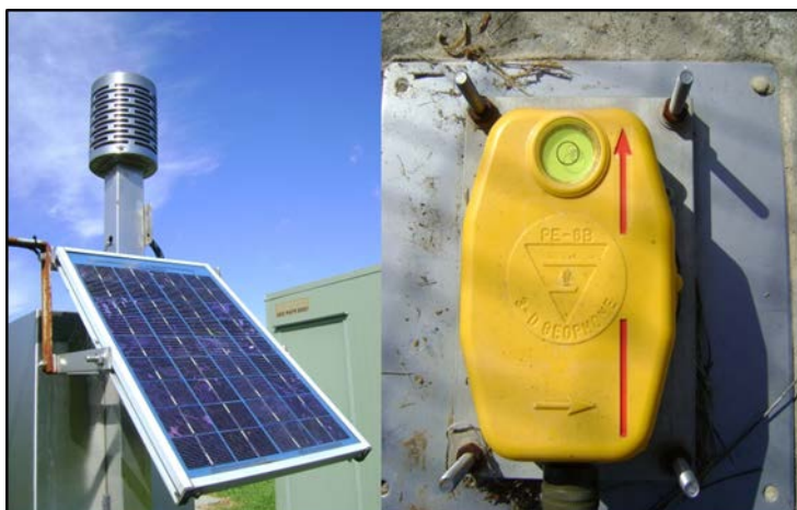
Figure 51 - BLAST MONITOR (microphone and geophone) AT QUEEN STREET (B1)
